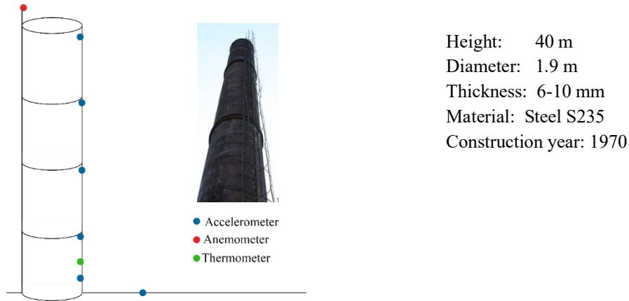
Figure 4.1. Installed monitoring system and information for the structure under study
