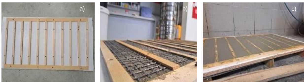
Figure 3. Preparation of the specimens (group II): a) moulds before lay-up procedure, b) embedding of fabric on the 1 st mortar layer, c) coupons prepared in molds
