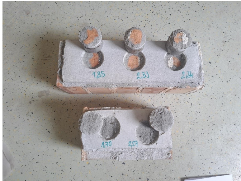
Figure 6. Brick specimens after the „pull-off“ test was done
