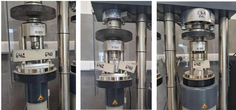
Figure 2. Testing of the mortar specimen
