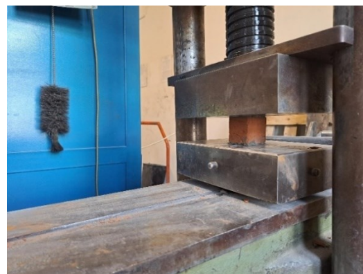
Figure 4. Preparation and testing of brick specimens
