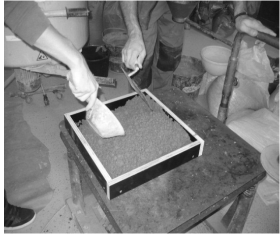
Slika 2. Ugradnja malterske mešavine u kalupe Figure 2. Embedding the mortar mixtures into molds
