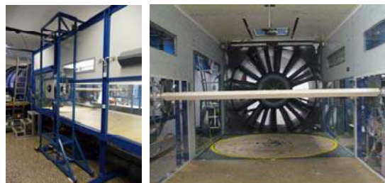
Slika 4. Model poprečnog preseka mosta postavljen na eksperimentalnu platformu Figure 4. Model of the bridge deck section placed in the experimental rig
