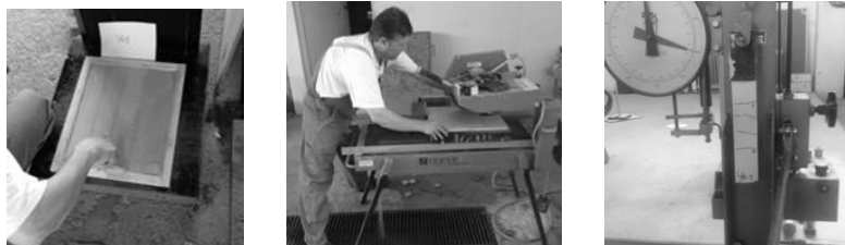
Slika 9. Testiranje jedne vrste FRCM sistema: izrada panela, rezanje, ispitivanje na zatezanje Figure 9. Testing one FRCM system type: production of panels, cutting, testing on tension
