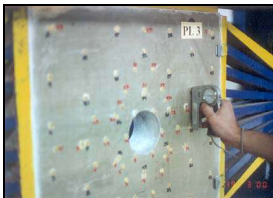
Slika 7. Mjerenje deformetrom tipa „Pfender“ na pločastom uzorku Figure 7. Measurement of deformations in plate specimen by deformer type "Pfender"
