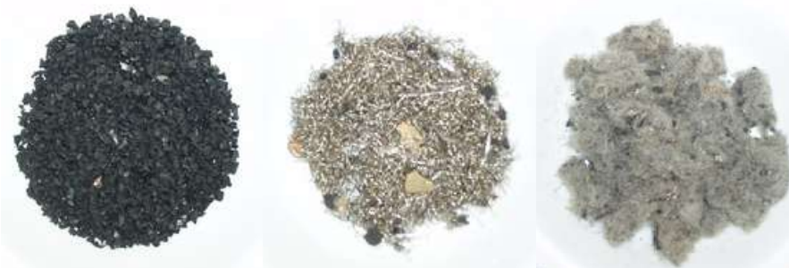
Slika 8. Guma, čelična i tekstilna vlakna dobivena reciklažom otpadnih guma Figure 8. Rubber, steel fibres and textile fibres from recycled end-of-life tires
