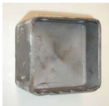
Figure 5. Lead-rubber bearings (LRBs, left) and Shear Panels made of mild steel (SPDs, right, specimen after pseudo-dynamic testing at the JRC Ispra) are usually the devices of choice for BI and HDS systems, respectively
